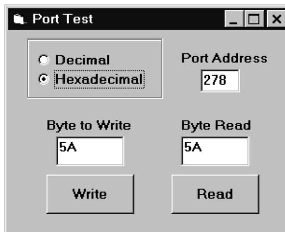
Figure 1. Use this Visual-Basic program to experiment with reading and writing to the standard parallel port and custom I/O ports.
