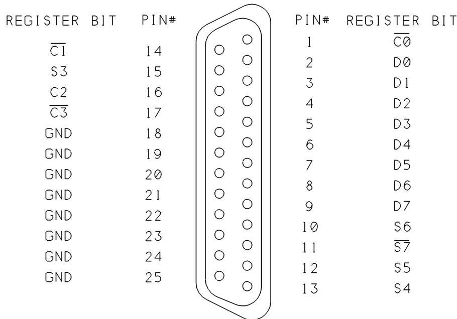
THE PARALLEL PORT'S 25-PIN D-SUB CONNECTOR AND SIGNALS
